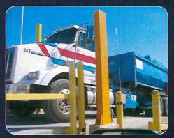
false alarm rate. If radiation signatures are present in a load of waste or scrap material, the system will immediately alarm and flash red to alert the user that a potential radioactive source has been detected.
